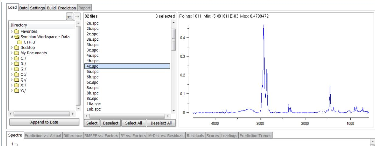
To select spectra for use by QT, simply highlight and select the desired files, or press “Select All”. Then press “Append to Data”. The display will now switch to the “Data” tab and the selected sample files will be listed. Here you can check any of the files that you wish to display.
