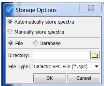
Pressing OK initiates data collection. We now enter the sample name and concentration values for the current sample. The example below shows a portion of the completed data table for our 82 samples. Here, we have chosen to display the current spectrum as well as two other manually selected spectra.
