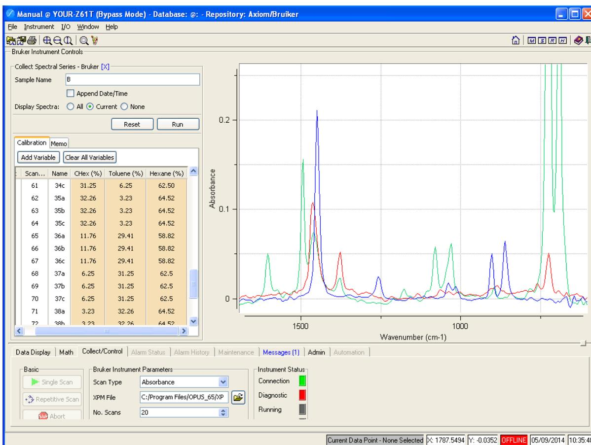
When we have completed the data collection process, we can exit the “Collect Spectral Series” mode by pressing the “X” at the top of the pane. The concentration values and other attributes will be stored in the designated location along with the associated spectra.
