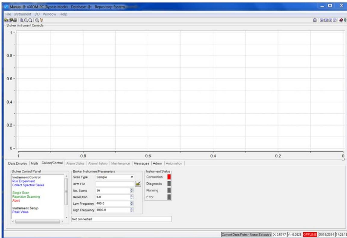
The panel at the left provides a selection of data acquisition choices. For the present illustration, we will select "Collect Spectral Series". The following pane appears.
