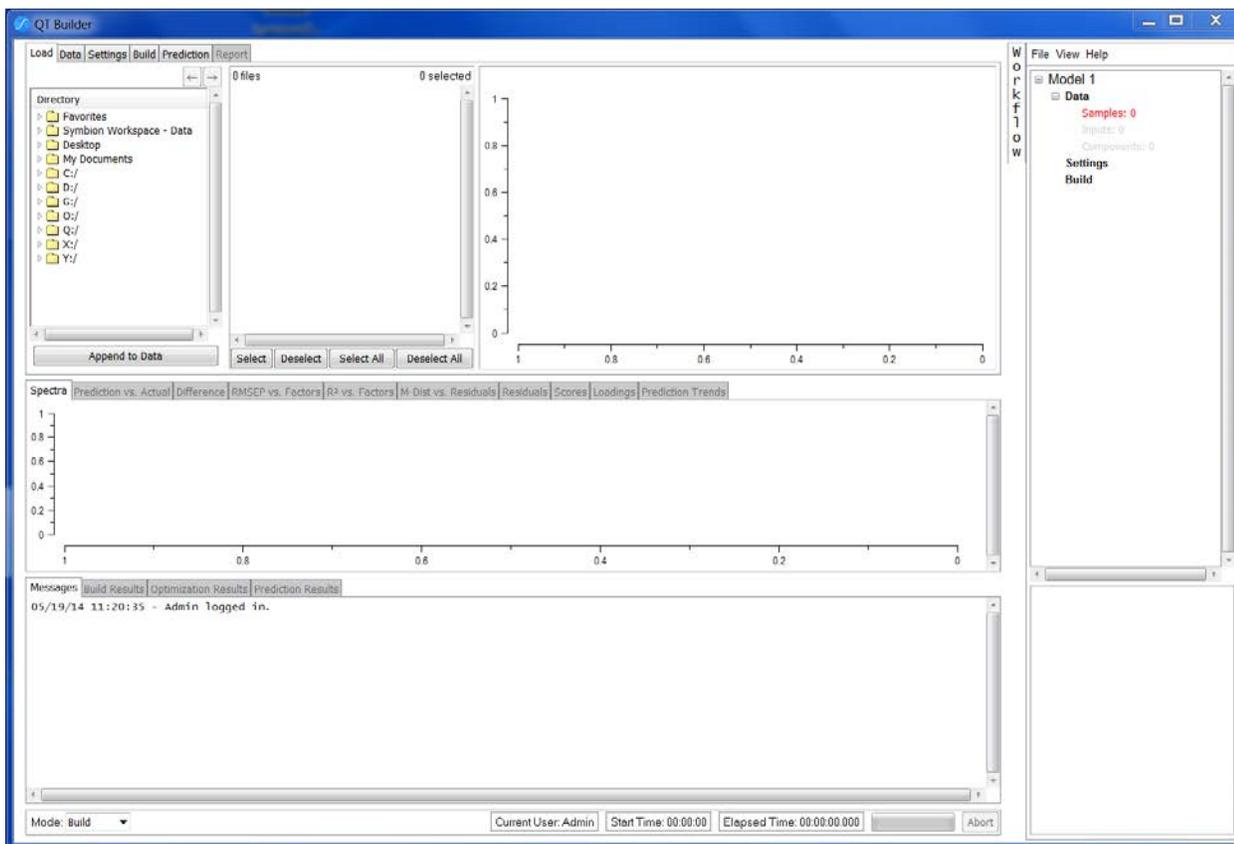
The first task is to load in the files to be used for calibration. This is facilitated by the navigation panel at the upper left. For our example (see below), we have navigated to the folder “CTH-3”, which was created during the data acquisition step, above. The list box shows all of the files that QT recognizes as data files, in this case 82 spectra. We can quickly preview any of the data in the folder by using the left click mouse function, as illustrated below.
