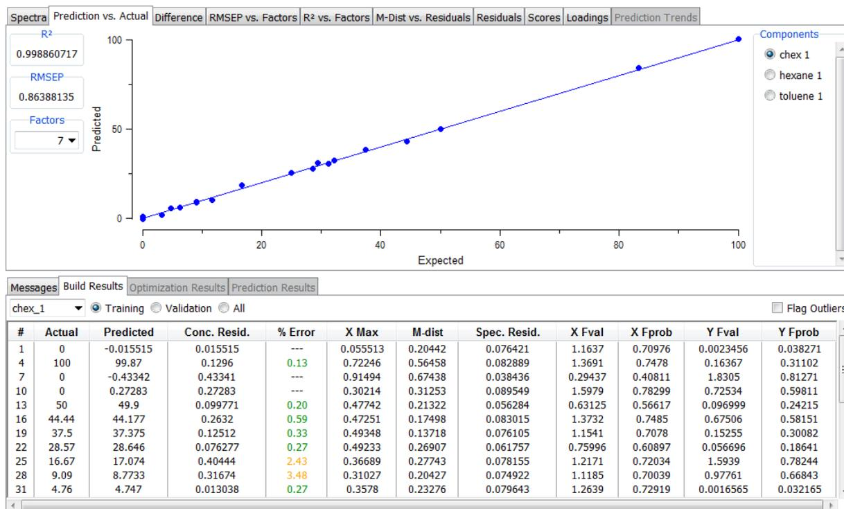
The user can check the goodness of fit by the level of linearity shown in the above plot. The percent error of prediction for each sample can be assessed in the lower pane. The percent error is color-coded so that the user can quickly determine which samples are outliers. The results shown are for cyclohexane. Checking on the other two components, in turn, will provide the corresponding results.
