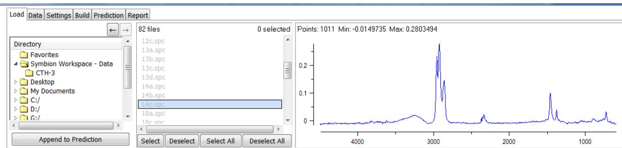
Next, select the desired data files or simply press "Select All". Then press "Append to Prediction". The program will then switch to the prediction tab and a list of spectra will be displayed. Next, we press "Predict" at the upper right. A table of predicted values and a set of prediction trend plots will appear.
