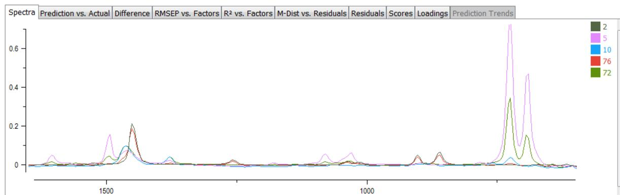
The identification of the chosen spectra is indicated by the color coded numbers at the right. The contributions of the successive factors to the goodness of fit can be evaluated by selecting either "R<sup>2</sup> vs. Factors" or "RMSEP vs. Factors". Since the latter is plotted on a log scale, it provides a more sensitive measure. In either case, individual plots are provided for each component.
